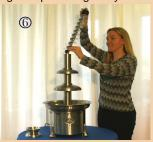
Step (7) Now place the crown on the top and your fountain is completely assembled. Set the temperature control to between 158 and 176 degrees. Turn the selector switch to start and watch the chocolate flow over the tiers. If the flow of chocolate over the tiers is not smooth and even, refer to the troubleshooting page for help and instruction.
